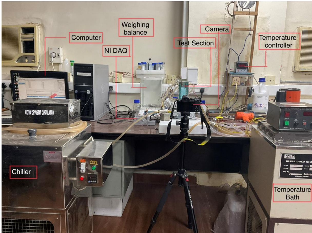
Figure #1: Experimental facility for nano-enhanced PCM based thermal storage systems
