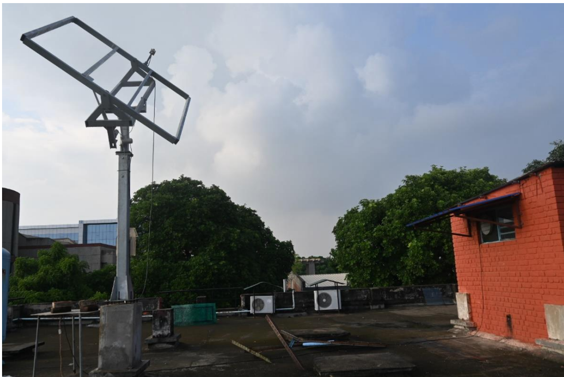
Figure #4: Two axis solar tracker for testing large scale panels
