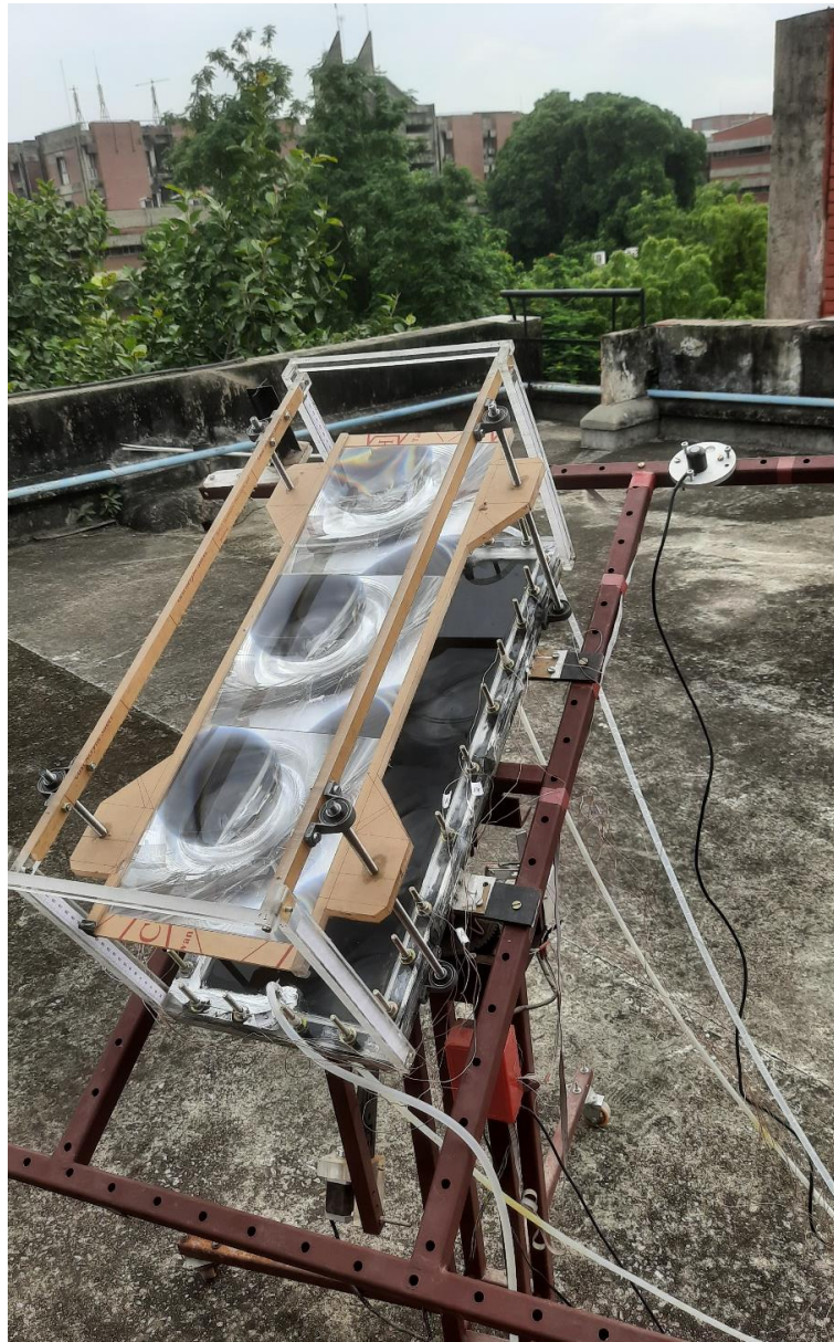
Figure #5: Solar desalination system based on Fresnel concentrators and nano-enhanced mebrane
